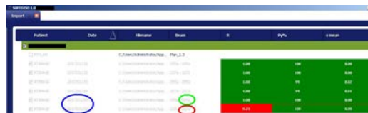
Figure. Figure shows a typical result after automatic synchronization. In green the test within tolerance levels in red the test out of tolerance. In this case, on 20 January 2017, you will investigate the R value for the field 227a and not for the field 055a saving time.
